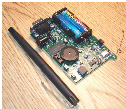
Figure 5. Prototype SpotON radio tag. These tags use radio signal attenuation to perform ad hoc lateration. Ad hoc clusters of tags cooperate to factor out measurement errors for all tag positions.
